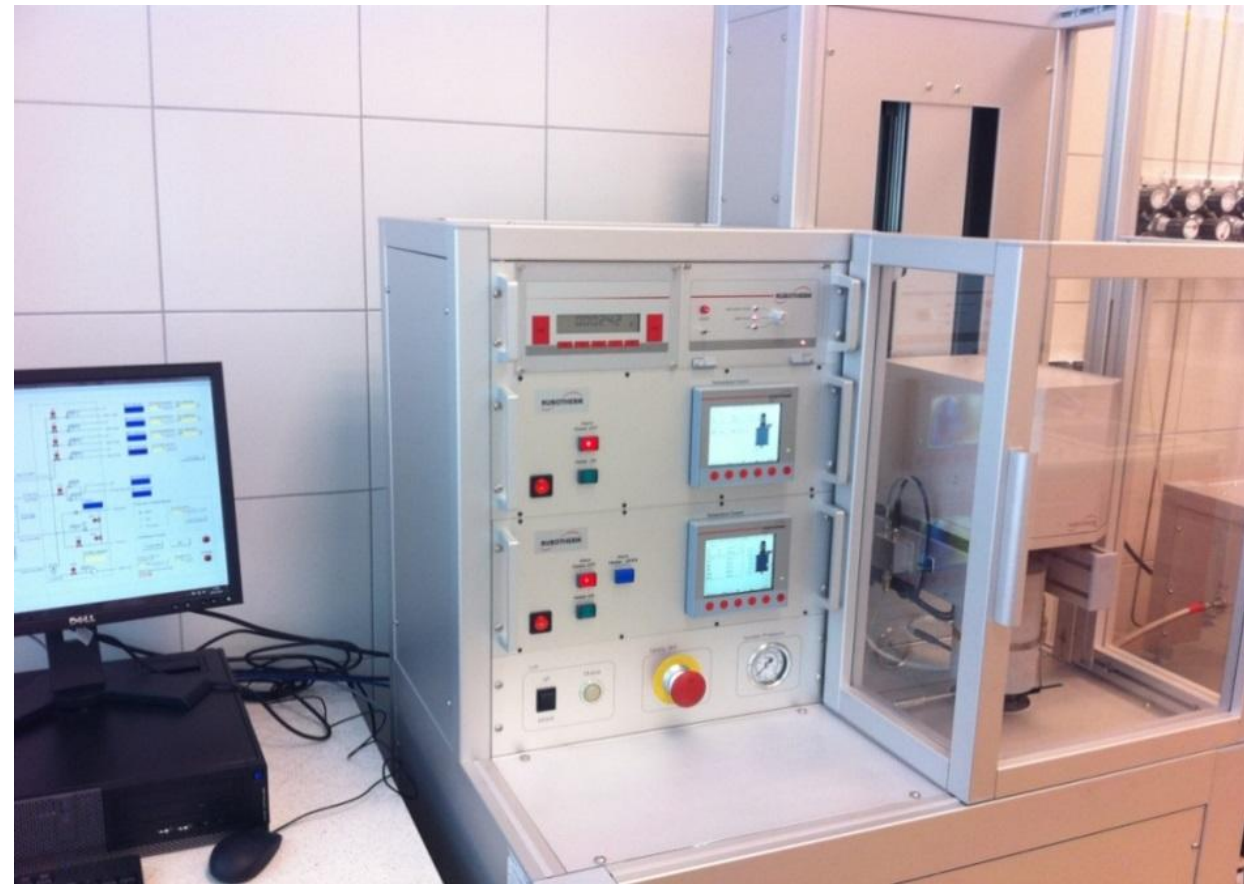
Fig. 1 High-Pressure Thermogravimetric Analyser (TGA) with MS
