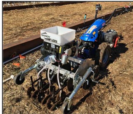
Powered coultter drill for walk-behind tractor: Kornecki et al., 2016, Patent Publication Appl.
