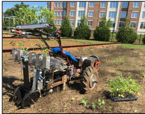
No-till transplanter for walk behind tractor: Kornecki et al.; 2018, U.S. Patent number: 10,004, 174 B2
