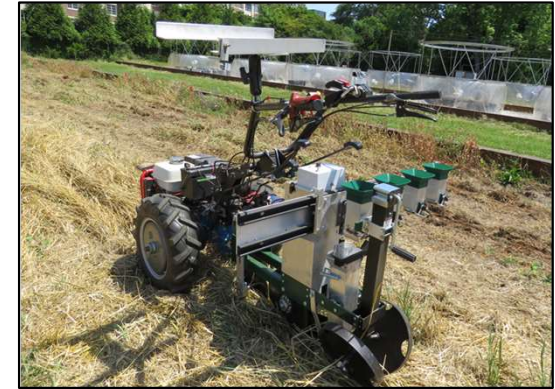
No-till transplanter for walk behind tractor: Kornecki et al.; 2018, U.S. Patent number: 10,004, 174 B2
