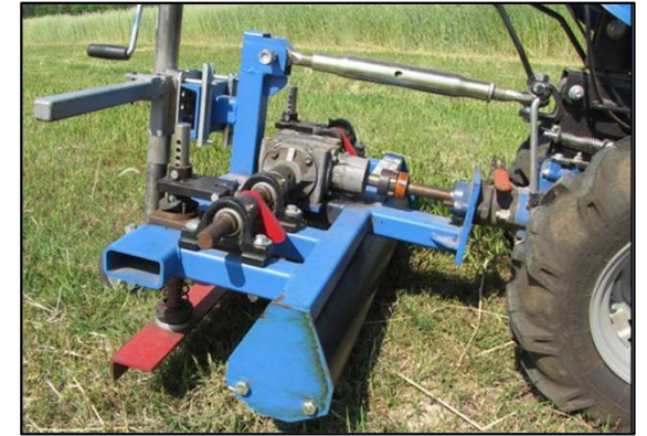
Powered roller/crimper, Kornecki 2012, U.S. Patent #8,176,991 B1
