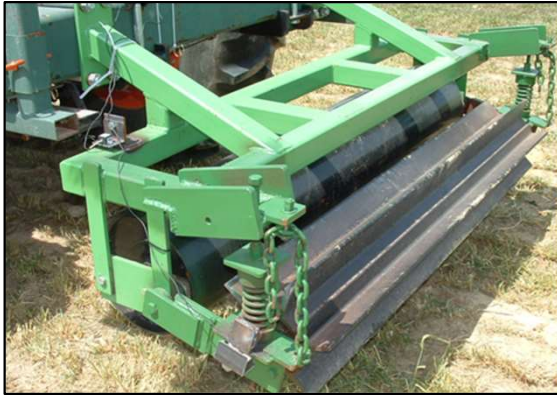
Two-stage roller/crimper: Kornecki, 2011 U.S. Patent #7,987,917 B1
