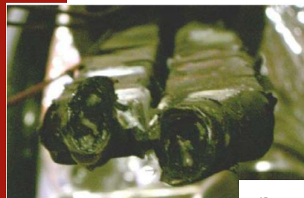
Figure 7: Model of resistive joint in bus bar with bad electrical and thermal contact with the stabilizer
