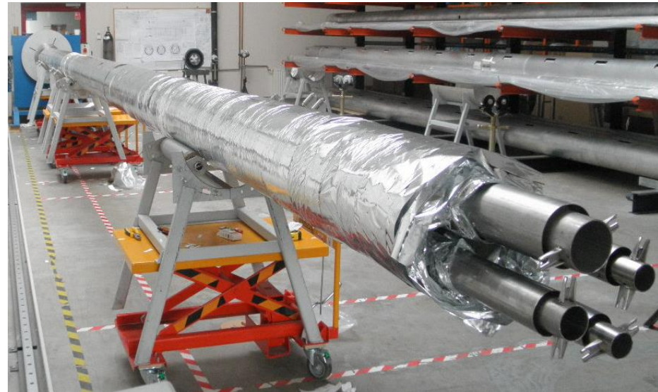
Winding MLI (30 layers) on the thermal shield (courtesy Kriosystem)
