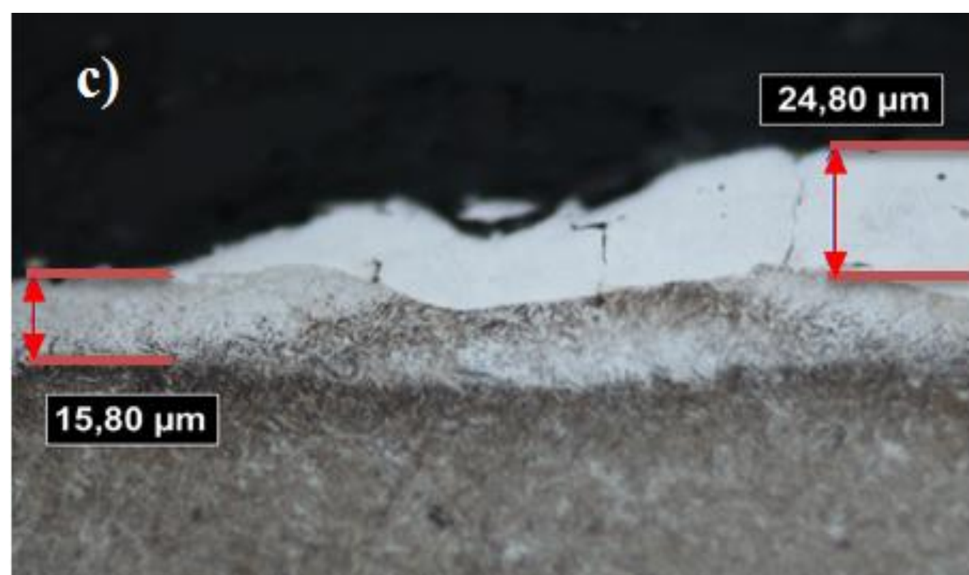
U = 25 \text{ V}, I = 8,6 \text{ A}, t_{on} = 200 \mu\text{s}, t_{off} = 11 \mu\text{s}
