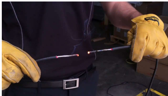
DC Solar Array - Arc fault demonstration, AC Solar Warehouse (YT)
